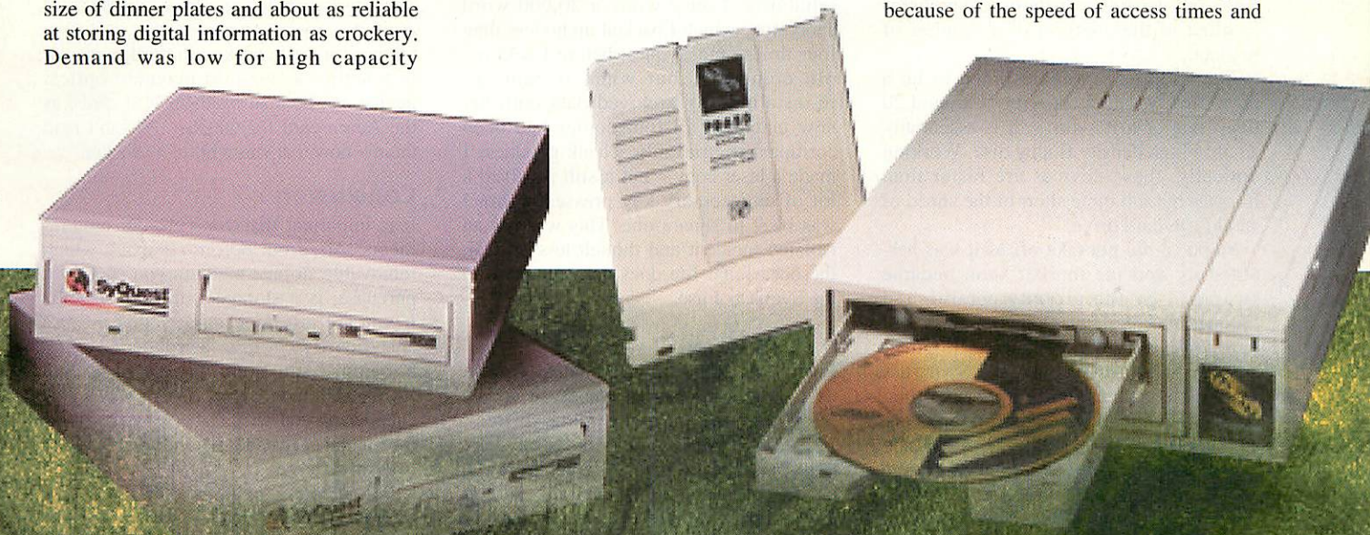
The shape of things to come? The Plasmon PD2000 CD-ROM drive will also write 650Mb phase-change optical cartridges.
